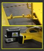
◆插入/卡入式牵引挂钩(选配)插入式成本低,但连接和分离不方便。 卡入式方便连接和分离,但是成本略高。 The cost of clevis coupler is low, but the connection and separation isn't convenient.
